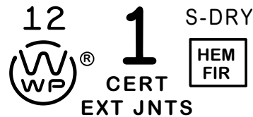
Fig. 2. Typical grade stamp for certified finger jointed lumber.
